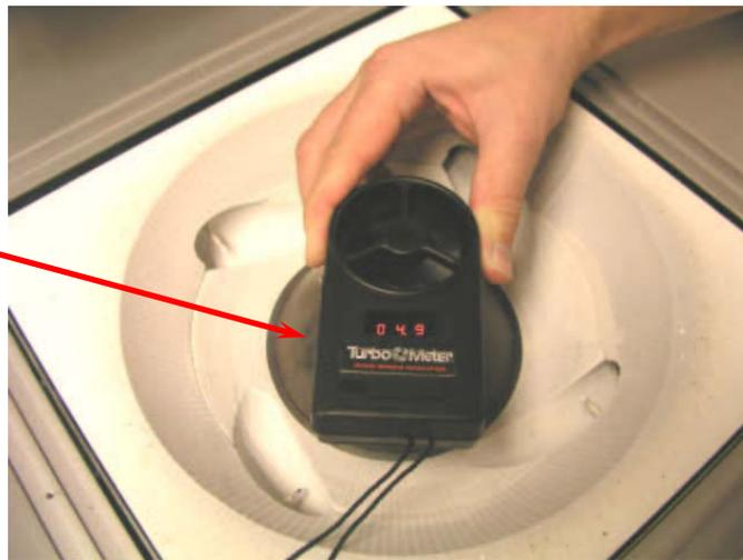
10. Vary the Bottom Heat (Preheater) Small airflow until the airflow setting on the Turbo meter reaches 5.0 knots. See below. When this is done, save settings. This completes small heater flow rate calibration.
