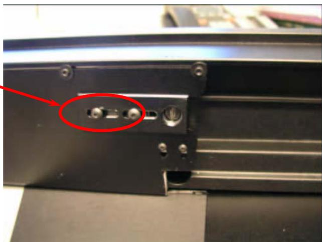
3. If the vacuum nozzle image is not centered in the software window in the X movement, remove the camera heat shield plate and loosen the four camera lock-down screws located underneath the front part of the camera. (Single camera version.)
