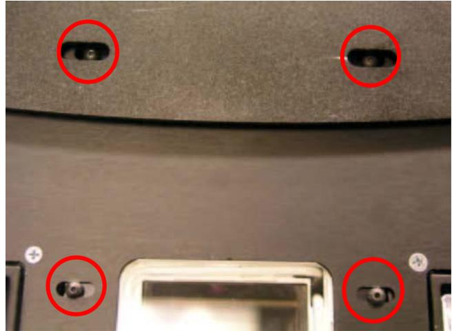
4. When loosened, adjust the X-axis movement as needed to align the vacuum nozzle image to the center of the software image window.
